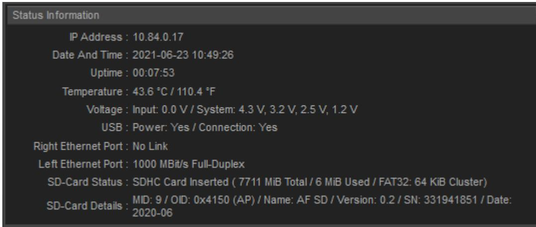
**IP Address** Shows the IP address set for the device as common identifier in Ethernet networks.
