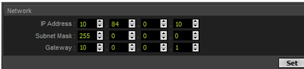
**IP Address** Is an identifier for devices that enables network communication. When using network protocols, it needs to be unique and set up for each individual sender or recipient in the network. Your MADRIX AURA already has set a valid IP address by default [for example, 10.84.0.10].
